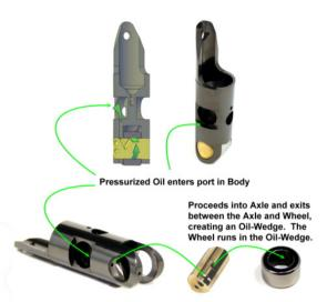
Recommended Spring Pressure 150-400lbs Seat Pressure 550-1000lbs Open Pressure
